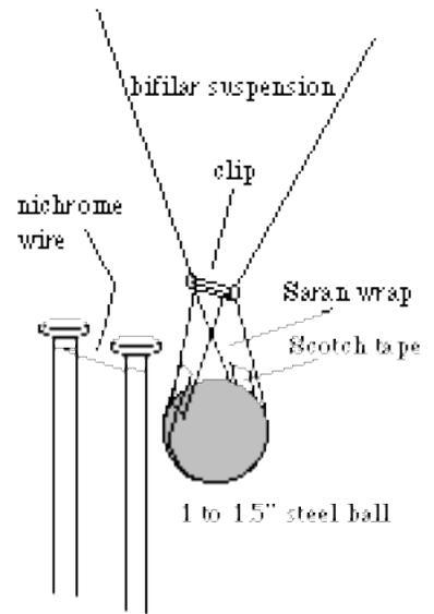
Begin by making the sling support for the steel ball projectile. Cut yourself a piece of Saran™ Wrap that is approximately 3/4" x 4". You will need several of such pieces throughout the experiment. The more consistent you are with the length of the suspension, the better your experimental results will be.
