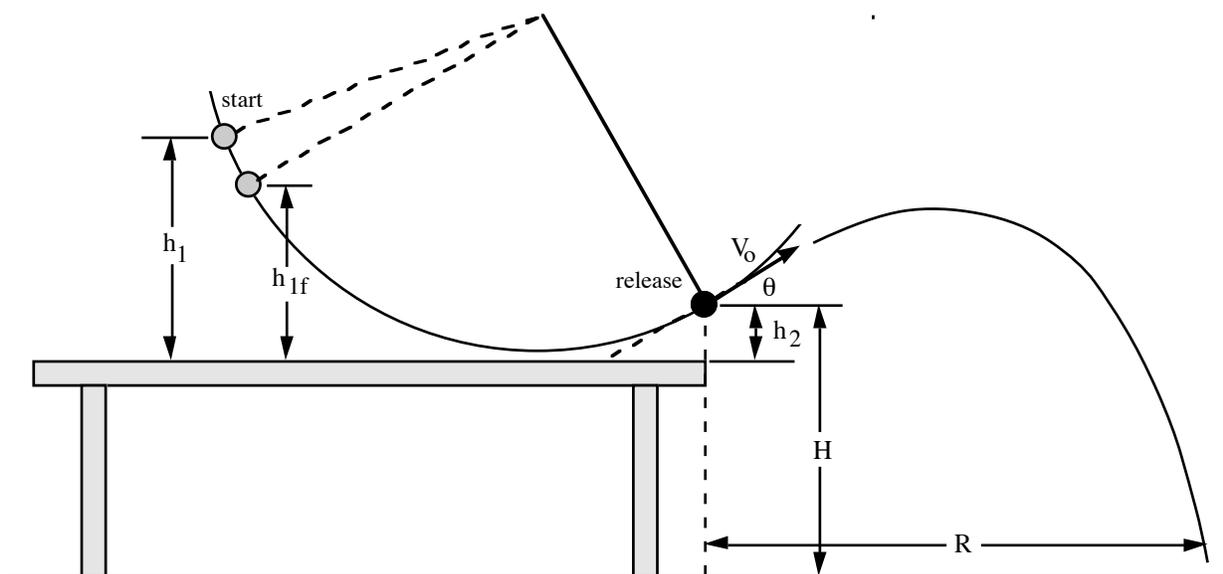
**Objective:** You will attempt to predict the range of the steel ball by invoking the law of conservation of energy to determine  $v_0$  and kinematics of trajectory motion to predict  $R$ .
