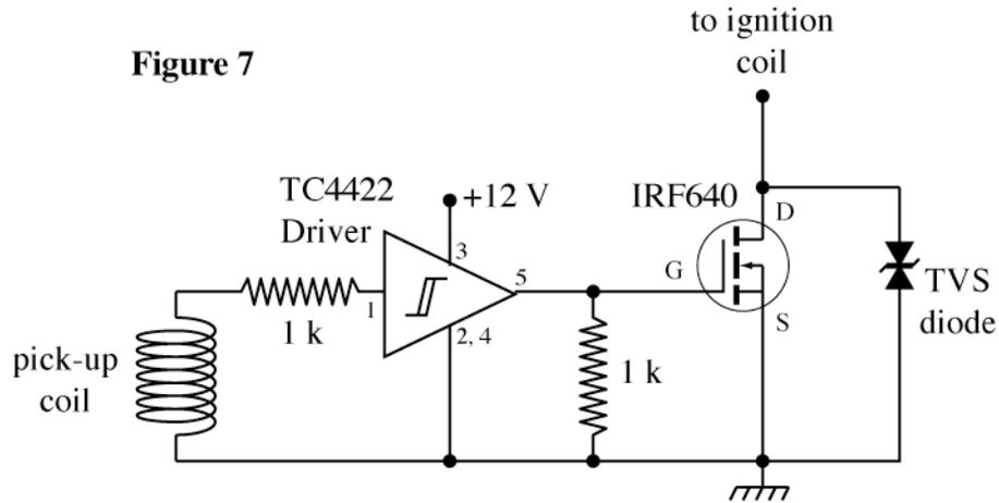
To help you navigate around the circuit board, Figure 8 shows the pinout configurations of the components. Although the IRF640 has an internal protection diode, the TVS diode has been added for double protection and is intended to shunt any transients over 200 V to ground.
