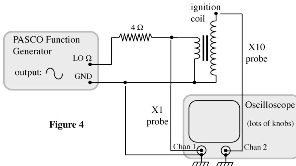
**11. How could you determine the turns ratio for your particular coil? Briefly describe what you would do to measure the turns ratio. Proceed with your measurement after checking with your instructor. What is the turns ratio?**
